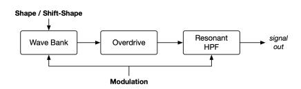
With a newly initialised patch, *unity* produces just a single oscillator with the *Shape* control morphing between triangle and sawtooth forms.
